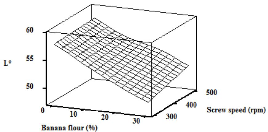
**Fig. 4 Effect of Screw speed and Banana flour on  $L^*$  value of fried extrudates.**
