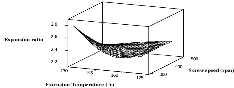
**Fig.6. Effect of extrusion temperature and screw speed on expansion ratio of extrudates**
