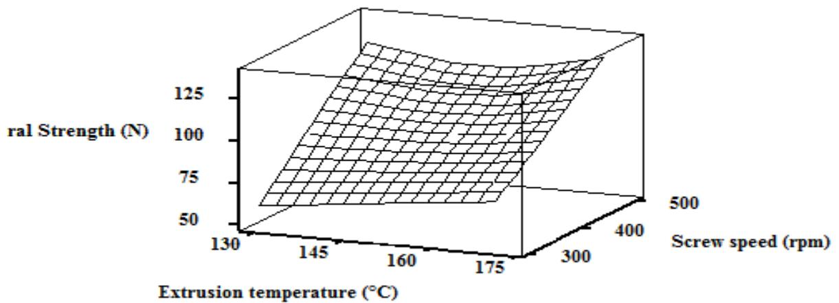
**Fig. 11(a) Effect of Screw speed and Extrusion temperature on Flexural strength**
