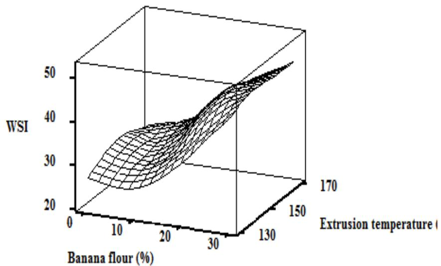
**Fig. 7 Effect of Banana flour and Extrusion temperature on WSI**
