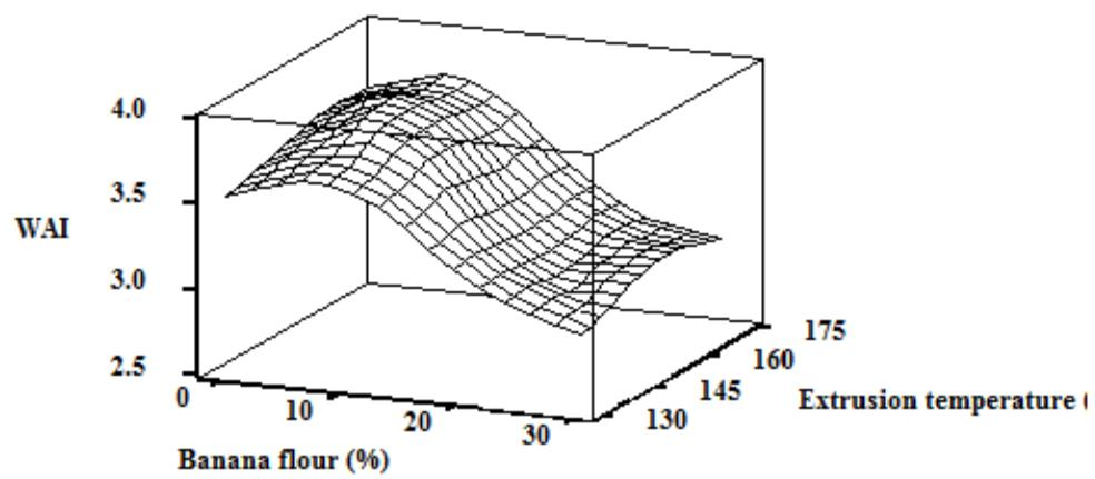
**Fig. 6 Effect of Banana flour and Extrusion temperature on WAI**
