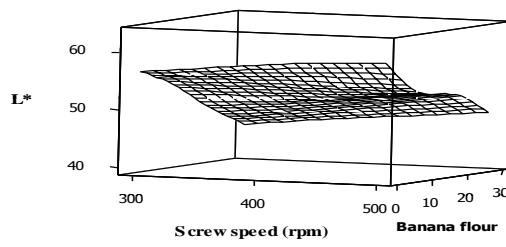
**Fig.3 Effect of screw speed and banana flour on the  $L^*$  values of fried extrudates**
