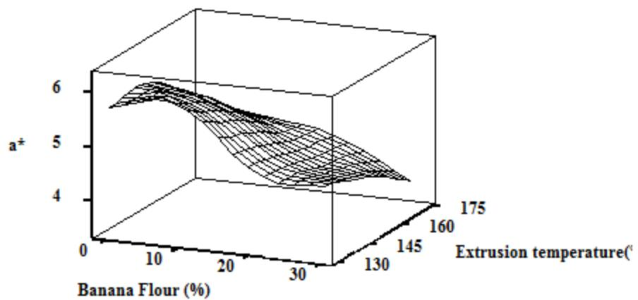
**Fig. 3 Effect of banana flour and extrusion temperature on  $a^*$  value of raw extrudates**
