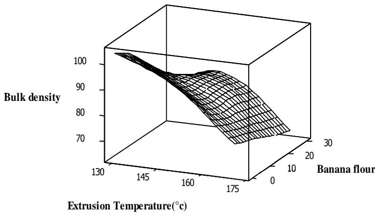
**Fig.5. Effect of extrusion temperature and banana flour on bulk density of extrudates**
